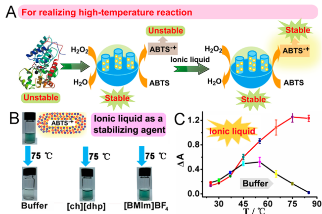
Figure 8. (A) Schematic illustration for the realization of high-temperature catalysis by using thermally stable EMSN-AuNPs and ionic liquid. 58 (B) Thermal stability of enzymatic product in different fluids. 58 (C) Catalytic activities of EMSN-AuNPs as a function of incubation temperature in different fluids. 58 Panels (A)–(C) reprinted with permission from ref 58. Copyright 2013 American Chemical Society.
